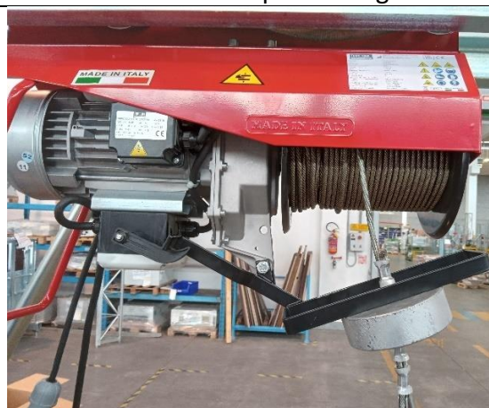
4 - Up stop lever, single-reeved model
