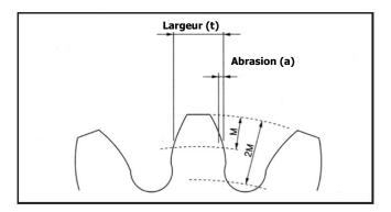
When the wear value reaches 0.15 t, it is time to replace the sprocket wheel.
