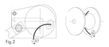
Never fit the rope in the opposite direction to the normal drum rotation indicated on the winch label. The friction brake would then be taken out of service.
