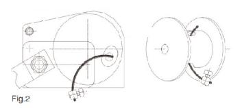
Never fit the rope in the opposite direction to the normal drum rotation indicated on the winch label.
