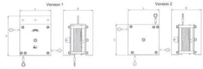
These load fall arresters ensure safety function in case of failure of the main loads holding or transporting systems.
